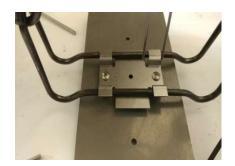
STEP 4: AT THIS POINT, YOUR TRAP SHOULD LOOK LIKE THE PICTURE. DOUBLE CHECK TO MAKE SURE THAT THE SAFETY LATCHES ARE STILL IN PLACE AND THE TRAP IS IN THE BRACKET WITH THE TRIGGER LOCATED AT THE TOP.
