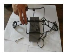
**STEP 3:** OPEN YOUR TRAP JAWS AND MOUNT THE TRAP TO THE STABILIZING PLATE AS SHOWN.
