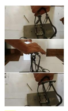
STEP 5: HOLDING THE TRAP WITH ONE HAND USE YOUR OTHER HAND TO SET THE TRIGGER. MAKE SURE YOUR TRIGGER LOCK IS IN THE MIDDLE SECTION OF THE TRIGGER SO THAT IT CAN LOCK PROPERLY.
